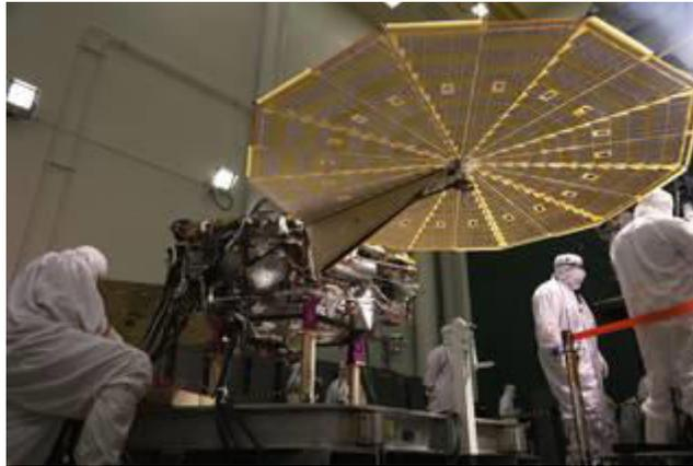
While in the landed configuration for the last time before arriving on Mars, NASA's InSight lander was commanded to deploy its solar arrays to test and verify the exact process that it will use on the surface of the Red Planet.
