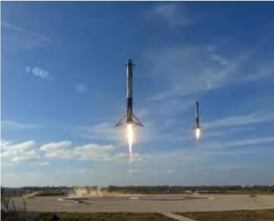
The three launch rockets returned to earth under power from most of their 27 rocket engines. The first two landed tail - down in Florida, and will be reused.
