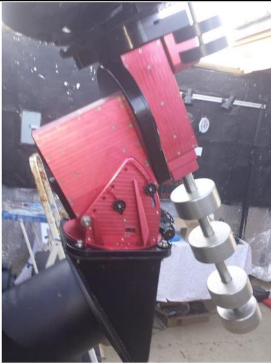
The RCX OTA weighs 70 pounds and requires two people to place it on the Paramount. My neighbor modified the pier by welding on a plate that mated with the Paramount base. The picture above shows the Paramount attached to the modified pier.
